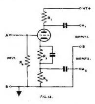
This takes advantage of the fact that a valve shifts the phase of the amplified signal 180 degrees. In other words, the signal in the anode circuit is opposite to the input signal and the signal in the cathode circuit has the same phase as the input signal.
