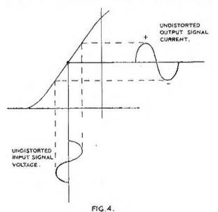
i.e. by applying a larger input signal voltage from the previous valve or pick-up device.
