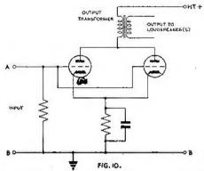
This is one method of doubling the power output by adding only one valve.
