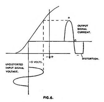
A Class AB<sub>2</sub> amplifier is biased to about the same point as a Class AB<sub>1</sub> amplifier, but when the effective voltage on the control grid becomes positive during the positive peaks of the input signal, distortion occurs and Figure 7 shows this relationship. You will notice that both the positive and negative parts of the signal are distorted.
