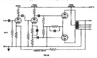
In order to improve the performance of amplifiers by reducing distortion in the signal and improving signal to noise ratio, part of the signal at the output is frequently connected to the input amplifier stage. This is called feedback and is normally out of phase with the input signal. In this case we call it negative feedback. Figure 16 shows a push pull amplifier with negative feedback.
