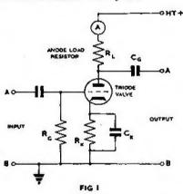
Figure 1 shows a typical triode amplifier. If we place an ammeter in series with the anode load resistor RL as shown in Figure 1, we can measure the current flow through the valve in milliamps. (Note: 1 Milliamp = 0.001 amp. or 1/1000 of an amp. and this current is known as anode current.) If we set up our circuit as shown in Figure 2 we can vary the voltage on the control grid by rotating the slider of P.1, and cause the anode current to vary with the grid voltage variations.
