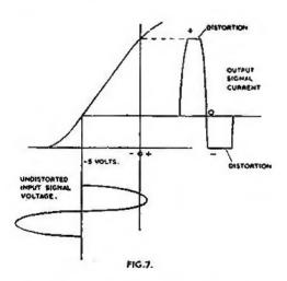
A Class B amplifier has the grid bias voltage set at the value where no anode current will flow. Figure 8 shows this type of operation.
