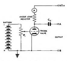
TEST CIRCUIT. IN THIS DIAGRAM A 12 VOLT BATTERY IS USED TO PROVIDE A NEGATIVE GRID BIAS VOLTAGE ON THE GRID OF THE TRIDDE VALVE, THE THICK GINES - THE NEGALIVE SIDE OF THE BATTERY(-) AND THE LONG LINES - THE POSATIVE SIDE(+) NOTE THAT THE + IS CONNECTED TO EARTH - BY MOVING THE SLIDER OF THE POTENTIOMETER P. WE CAN VARY THE VOLTAGE WHICH APPEARS ON THE GRID OF THE VALVE, R., IN FIGURE I REPLACES THE BATTERY SHOWN IN FIGURE BUT IT DOES THE SAME JOB.
