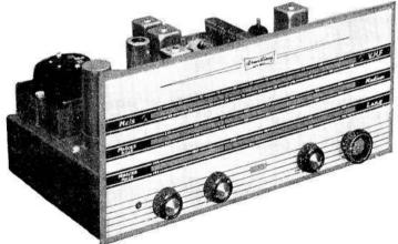
ST3 Mk2 AM/FM TUNER 27 gns. This new tuner is the successor to the welltried and successful ST3. Improvements in design and a considerable reduction in size make the new tuner even more attractive than its predecessor. It includes all the features of the T4 tuner and the A.M. section covers the long and medium wavebands. The ferrite aerial and unique 2nd I.F. stage ensure good continental reception and there is a miniature bright-line indicator for easy tuning.
