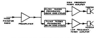
FIG. 1. SPLIT AMPLIFIER FREQUENCY DIVIDING SYSTEM GIVES GOOD LOUDSPEAKER DAMPING
