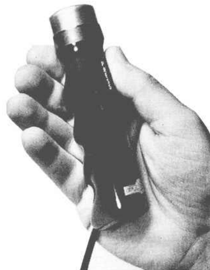
Fig. 5. The Lustraphone LH/59 magnetic moving-coil hand microphone.
