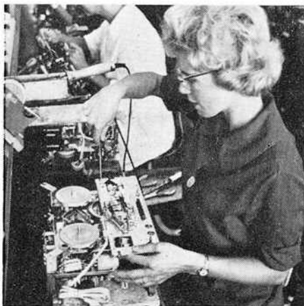
A final stage in assembly before the deck cover is fitted.
