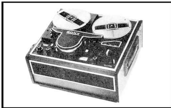
Fig. 7. The new Sony video tape recorder employs a tape speed of 7\frac{1}{2} ips and a rotating head record/playback system.
