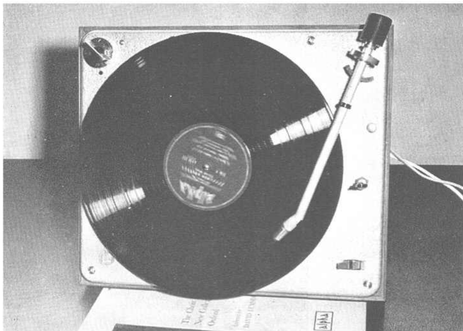
Fig. 3. True picture showing the unit actually tracking at about 2 gram at 33½ rpm in an almost vertical position.
