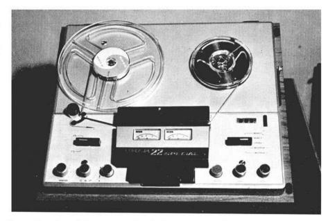
Fig. 5. Top view of the recorder with plastic cover removed.
