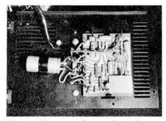
Fig. 6. Close-up of one channel power amplifier section.
