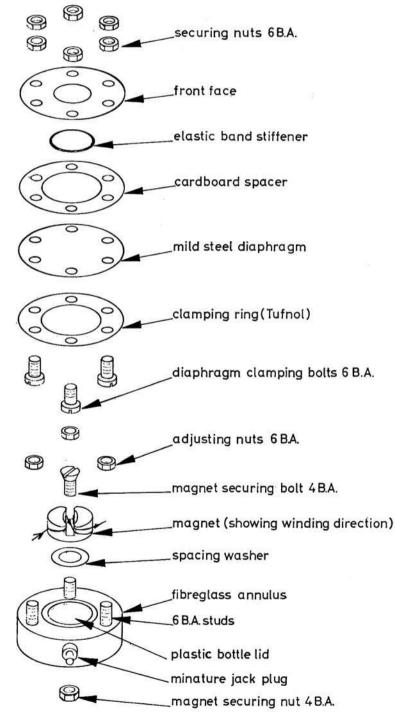
Fig. 2 Exploded view
