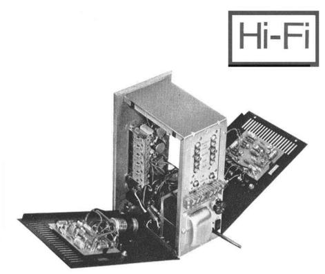
Fig. 4. Showing the amplifier de-boxed and with the power amplifier side sections hinged down.
