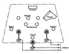
Fig. 2. Careful placement of the microphones is necessary for a group of instrumentalists.
