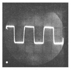
Fig. 6. Square-wave through amplifier at 2,000 c/s.
