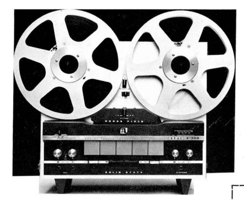
The Akai X 300 is a 4 track stereo/mono studio-type tape recorder. It has 4 heads – erase, record, playback/monitor, and Crossfield; and 3 motors – one hysteresis synchronous direct drive capstan, two torque for fast forward and rewind. It has two speeds –  $3\frac{3}{4}$  ips which will give you 30 to 18,000 cps  $\pm$  3db; and  $7\frac{1}{2}$  ips which will give you 30 to 24,000 cps  $\pm$  3 db.
