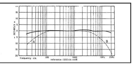
Fig. 2. Frequency response characteristic. Taken across 8 ohms at 0.5 W, tone controls flat and filters out. (A) shows the effect of If filter and (B) the effect of hf filter.
