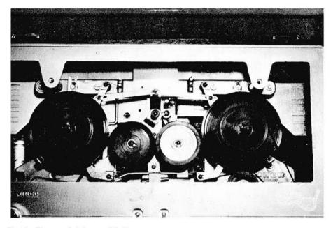
Fig. 4. The spool drives and belts.
