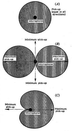
Fig. 1. Polar responses of microphones: (A) Omnidirectional, (B) Bidirectional, (C) Unidirectional (cardioid).
