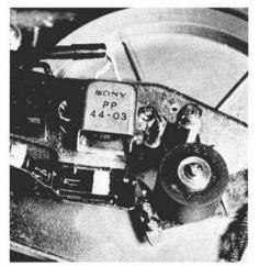
Fig. 3. Head adjustment on Sony recorder.
