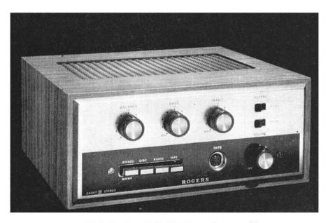
Fig. 2. The Rogers Cadet Mk.3 integrated stereo amplifier.
