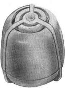
Specification: Moving-coil Model LD 61, medium impedance (nominal 600 Ohms at 1 kc/s) in cream plastic casing with a fabric blast guard, 9 ft. co-axial lead which can be extended to considerably greater lengths, fitted with a Belling-Lee coaxial plug—list price £3 7s. 6d., yours for only 26s. This high quality mic. is omni-directional in the horizontal and approaches cardioid characteristic in the vertical planes. Frequency response approx. 70-12,000 cycles/ sec. Sensitivity approx.-75 db (m).
