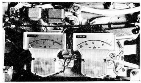
Fig. 1. View of head and capstan section with top cover removed, showing the twin recording level meters.
