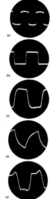
Fig. 7. Square wave performance. (a) 120 c/s test, (b) 2,000 c/s and (c) 10,000 c/s test, all with tone controls flat and filters out and signal to 'flat' input. (d) 2,000 c/s square wave signal to equalized input, showing RIAA compensation effect and (e) 2,000 c/s square wave, showing the effect of the hf filter.
