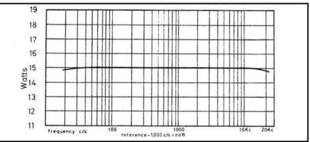
Fig. 1. Power response characteristics with tone controls flat, filters out, both channels operating simultaneously and power across 8-ohm load.
