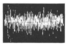
Fig. 1. Narrow band noise signal.
