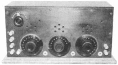
FIG. 5—DETECTOR AND TWO STAGE AMPLIFIER. THIS SET HAS AN EXTERNAL POTENTIOMETER ON THE DETECTOR TUBE. ALL OF THE REGENERATIVE SETS MADE AFTER THIS ONE HAD THIS TYPE OF CONTROL.
