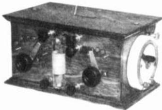
FIG. 1—THIS IS A AUDION CONTROL BOX DESIGNED FOR USE WITH A DOUBLE FILAMENT TUBULAR AUDION TUBE. IT RESEMBLES THE DEFOREST RJ-4 EXCEPT THE DEFOREST USES A ROUND TUBE AND THIS ONE THE TUBULAR AUDION. (PHOTO ALSO ON FRONT COVER OF THIS ISSUE.)
