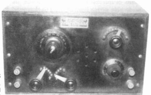
FIG. 7—A ONE TUBE REGENERATIVE SET USING A TUNING CONDENSER AND A TAPPED COIL. THIS SET WAS TYPICAL OF HIS STYLE, WITH THE DOOR OPENING IN THE REAR AND THE EXTERNAL POTENTIOMETER.
