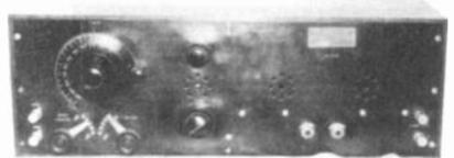
FIG. 9—THIS SET IS DESIGNED FOR USE WITH DRY CELL BATTERIES AND IS INTENDED TO USE THREE 199 TUBES. THE CIRCUIT AND CABINET IS BASICALLY THE SAME AS FIGURE 8.
