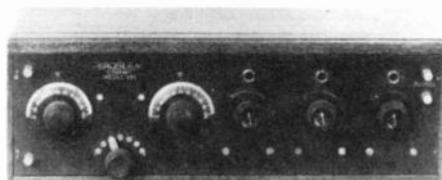
**MODEL VIII**-Crosley's Model VIII (eight) was a 3-tube receiver with one stage of tuned radio frequency amplification, detector, and one stage of audio frequency amplification. It was tuned with two wood-type book condensers and a cylinder style coil tapped seven times. In 1923 this set sold for \$99 and Powel included the works...(batteries, phones, and tubes).
