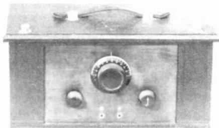
**MODEL SR4** - In 1925, Crosley made this one-tube portable exclusively for Sears. It was called the SR-4. Captured screws on top released the hinged lid to reveal an ultra-simple circuit using Crosley's latest variable-plate tuning condenser, black molded socket and rheostat. The leatherette covered case would hold the dry-cell batteries and phones. Phone pin holes were panel-mounted. A deluxe version used a brass-plated vernier tuning dial.
