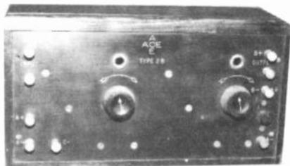
**ACE 2B** - The Precision division of Crosley made its own two-step amplifier to boost reception of the Ace V model one-tuber. It was called the "Ace 2B" and was exactly like the Crosley Model IV (four) amplifier. (Photo courtesy of Larry Wright)
