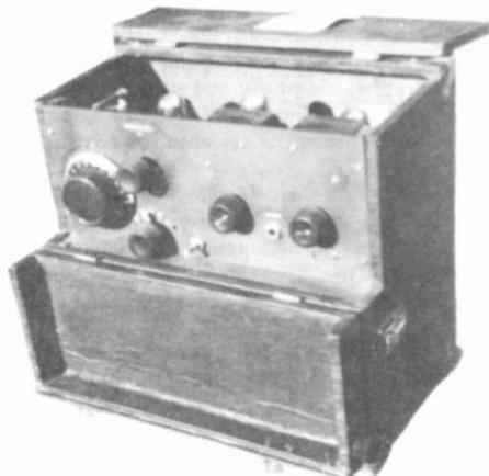
**MODEL 52-P** - Like the 51, the Model 52 three-tube receiver was marketed in a portable version. The black leatherette case was slightly larger than the 51-portable, but similar in design. Not many of this model seem to exist. Noticeable is the absence of panel binding posts, for they are moved inside to a bakelite strip behind the tube sockets.
