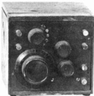
**MODEL SR-2** - The smallest Crosley regenerative receiver in a wood cabinet was this "SR-2" one-tube set. It was sold thru Sears and Roebuck exclusively and in actuality was the Model 50 squeezed so compactly that the panel of the Model 50 had to be rearranged. It was offered to the public for \$23.25 and aimed at the youth market.
