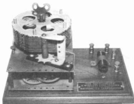
**THE NATROMETER** - This code teaching machine, like the Omnigraphs of its time, was a device that could generate random code for the purpose of instruction or testing by a mechanical wheel. It was wound up like a clock, and by the selection of any or all the removeable pins on top of the drum, pseudo random code would be transmitted to a sounder or buzzer. *Courtesy R. Rees.*
