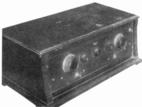
**NEWPORT TYPE 1112** - The more expensive Trirdyns were housed in more elaborate cabinets like this Type 1112 Trirdyn Special "Newport" that sold for just over \$100. The later Trirdyns panels were slightly redesigned to have the three center knobs align (both rheostats were raised) and the on/off switch moved to the left. Other Trirdyn models had names like "Standard", "Regular", "Biltmore" and "Super".
