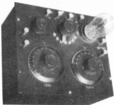
**PRECISION** - A set of mysterious background was this one-tube set of "Tri-City" design. It was sold under the Precision name and was the only Crosley set to ever use the wooden vario-coupler he manufactured. The tube socket was of "Ace" design. The rest of the parts were Crosley. This set might have been produced so Crosley could use up old parts.
