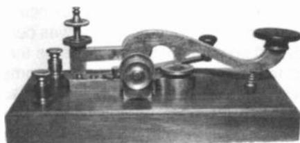
**KNOX & SHAIN CAMELBACK** - This 1870's vintage key has a style of its own. Of post Civil War making, it is a good example of the fine art of making camelbacks, soon to be phased out in favor of the straight, steel lever keys. It is made of heavy brass, and seems to have been part of a set. *Courtesy G. Potter.*
