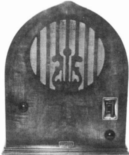
**ECHOPHONE** - Model "C"; this early cathedral dates around 1929-30. With the uses of 01A tubes and a front panel mounted regeneration control, this set is a good example of the "Midget or Cathedral" evolution. The six tube chassis is mounted on the back of the cabinet using the following tube line up: 01A's for the first and second RF and first audio, a 27 for the detector, a 71 for the output and an 80 for the rectifier. (*John Miller - Lexington, KY*)
