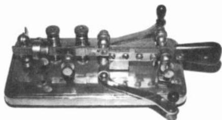
**THE SEMATIC BUG** - This Signal Electric bug could be used as either a speed key, or by closing both shorting bars and flipping over the catch at the end of the operating pendulum, it could be used as a sideswiper. This model is nickel plated and about a third larger than the black based models. They were made in the late 1920's. *Courtesy C. Hinkle.*
