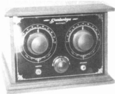
**STANDARDYNE** - A very unique set using a "multivalue" tube (three tubes in one glass envelope), it was made in 1925 by the Standard Radio Corp. of Worcester, Mass. The sloping front panel is housed in a nice walnut cabinet, measuring 11 $\frac{1}{4}$  inches wide, 9 inches deep at base, and 8 inches high. A very desirable set with collectors, this radio is quite scarce, and needless to say, the vacuum tube is almost as difficult to find as the radio itself. (Gary Schneider - Cleveland, OH)
