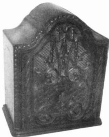
**WHAT IS IT?** - This set features a Repwood front and solid wood sides. Uses the following tubes: Three 24's, one 27, one 45 and an 80 rectifier. The 24's are highly shielded. This broadcast band set was probably made in the early 30's. Looks as if there was some kind of decal on the inside of the cabinet at some time. Anyone have knowledge of this radio? (*Andrew Mooradain, 5 Priscilla Lane, Winchester, MA 01890*)
