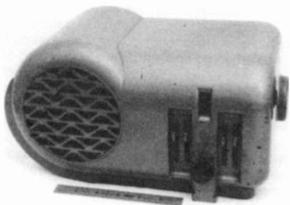
**STEWART-WARNER - Model 97-573** ("Varsity") made in 1939. Metallic light blue finish on bakelite. Five tube AC-DC circuit with mechanical push button tuning. I would call this design & color "Art Yetcho"! (Robert Lozier, Monroe, NC)
