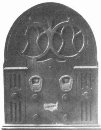
**INTERNATIONAL** - 1931 "All Wave Duo", also sold under the Emerson and Acratone names. Two discrete radios in one, the set featured both broadcast and shortwave reception. The Duo had separate tuning condensers, dials, and controls on the same chassis. Uses 8 tubes - 2-24A's and 27 in shortwave circuit (Superhet) and 2-35's and 1-24A in broadcast circuit (TRF). (Bill Moore - Huntsville, AL)
