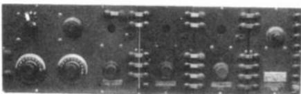
**NORTHERN ELECTRIC - This R-1** is a one-tube regenerative detector using a 215-A peanut tube designated R215-A in Canada. It is shown along with two R-5 audio amplifiers (also each with one R215-A), and a R-105 loudspeaker amplifier using a R216-A tube. The R-1 probably appeared about 1922, but its most recent patent date is 1919. Total price \$133.50. (Bob Murray - Winnipeg, Manitoba)
