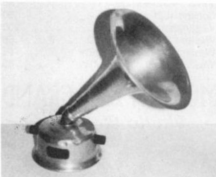
**MOON** - Unusual speaker manufactured by the Wilson Utensil Co. of Dayton, Ohio. Made of aluminum, it is 15 inches tall and has a bell diameter of 10 inches. Headphones were placed on the two projections sticking out of the base and were used as the driver. (*Rudy Burick - Parma, OH*)
