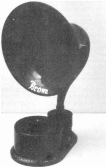
**E.G. BROWN CO.** - This Brown's Crystavox horn speaker has a built in carbon granule "amplifier"; just connect up a battery and you can listen to your crystal set. Made by S.G. Brown Co. in England, circa 1925. (*Alan Brehaut - Timaru, New Zealand*)
