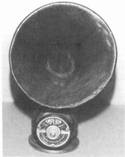
**AMPLION** - This small speaker stands 8 1/2" high and the bell of the horn is 5 1/2" in diameter. Two binding post on top of driver unit are for wires to receiver (not shown in photo). Tone/volume adjustment is on front of driver. Front plate reads "Amplion Loud Speaker - Type AR 102". The casting which holds the driver and attaches to the horn is imprinted on the back "Made in Great Britain". (*David McKenzie - Eustis, FL*)
