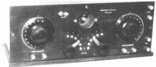
**GREBE CR-3A** - This scarce set uses two wood variometers and has the detector tube mounted on the front panel. The set has no filament rheostat so one must be connected externally. Also, it uses a Cherry cabinet, not Oak. Made in late 1920. (Previously owned by: Jerry Finamore - Budd Lake, NJ)
