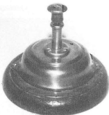
**PREECES PLUNGER KEY** - This oddity was made in Britain and is mounted on a six inch diameter wooden base. The keying mechanism inside is exactly like the precision made Post Office design keys made during this period. It has a great feel, and was probably used in railroad signaling about 1910. *Courtesy T. Shedd.*
