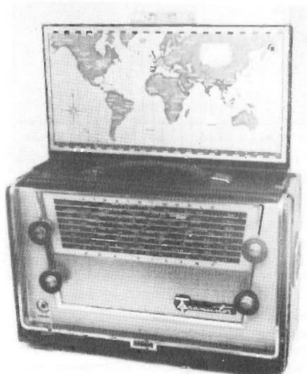
**RCA VICTOR** - All transistor "Strato-World", model 1-MBT-6, of 1956/57. Loop built into flip-up front cover. Seven bands, TRF front end - very "hot", good audio quality. Uses nine D cells. About the size of a Transoceanic. (Robert Lozier, Monroe, NC)
