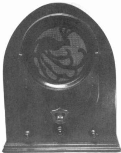
**JACKSON-BELL MODEL 62 (ART DECO):** There were some other shaped cabinets in this model per Frank Heathcote. It has two interesting screw-in copper capacitors with one top lead each, copper socket being ground. (G. Hauske - Wheaton, IL)
