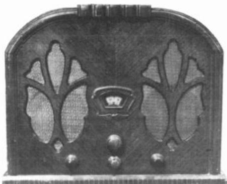
**STEWART-WARNER MODEL R-110-AT** - Manufactured by the Stewart-Warner Corp. of Chicago. A ten-tube dual wave superhet covering 75-550 meters, it sold for \$49.50 in 1933. Among its features are two 4-inch speakers, automatic noise suppression, push-pull resistance, coupled output tubes, and AVC. (Frank Heathcote, Logansport, IN)
