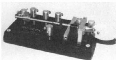
**GO-DEVIL BUG** - This was designed to be used as a regular bug but would also double as a keyer paddle or sideswiper when the damper arm is latched into a fixed position by the catch on the damper mechanism. Notice the three terminals instead of the usual two. It is made entirely of aluminum except for plastic paddles. *Courtesy Phil Shafer, W7BM.*
