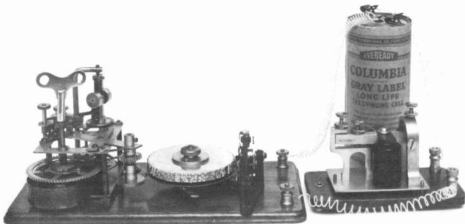
**OMNIGRAPH** - Code practice machine of 1915-20 vintage. Accepts 5 code discs that could give 100 different character groups when various combinations of the four levers were set under the code disc turntable. Later versions could accept 15 code disc. Shown with Menomonee six-ohm sounder (Robert Lozier - Monroe, NC)
