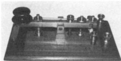
**MARCONI WIRELESS TELEGRAPH CO.** - Spark key on a wooden base. Notice the original extra pair of contacts that short out the coherer when the key is transmitting. It dates from 1910, and was an early attempt to upsize ordinary wood base landline keys for spark transmitters. It was found that the heavy currents would heat up the contacts and eventually char the wood leaving the keys mechanically unstable. Later versions used slate or marble for the base. *Courtesy Paul Giganti, W6GVY.*
