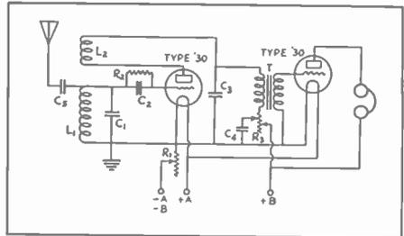
*A Type 30 regenerative detector circuit followed by a Type 30 audio-frequency amplifier similar to the type that David Brooks must have built. It even was to be built on a pine board! This circuit diagram is from page 61 of the Ninth Edition of the "Radio Amateur's Handbook" © 1932 by the American Radio Relay League. (Editor)*
