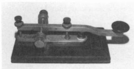
**LARGE SPARK ERA KEY** - Made by the American Marconi Co., this key is mounted on a slate base and has 1/2 inch silver contacts. It is of a similar size and construction to the United Wireless Co. keys of that time, one of which is on display at the AWA Museum in N.Y. *Courtesy Ralph Muchow.*
