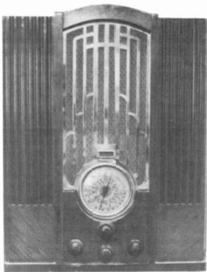
**ZENITH MODEL 334A** - An impressive ten-tube all-wave set covering 530 kHz to 46 MHz. Manufactured in 1934, it sold for \$89.95 and is a first class performer. The chassis was also available in a console cabinet. From the Jim Shirreff collection. (Frank Heathcote, Logansport, IN)
