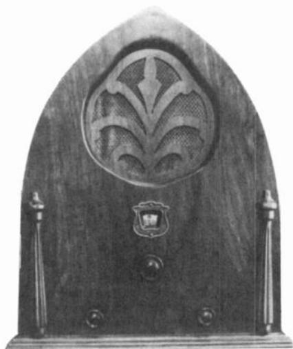
**ZANEY-GILL "MUSIC BOX" MODEL 2445** - A six-tube TRF set introduced in late 1930. Believed to have been manufactured by Electrical Research Laboratories, Inc. (ERLA) of Chicago, for the Zaney-Gill Corp. of Chicago and Los Angeles, a pioneer manufacturer of midget radios. (*Frank Heathcote, Logansport, IN*)
