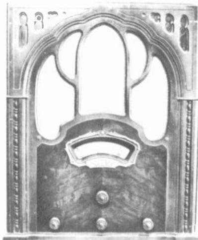
**U.S. RADIO MODEL 9A -** Manufactured by the U.S. Radio and Television Corp. of Marion, Indiana. A nine-tube superhet covering the broadcast band only, it sold for \$52.50 and was introduced in mid-1932. (Frank Heathcote, Logansport, IN)
