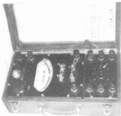
**TEST INSTRUMENT** - French wattmeter with current transformer in walnut case. Very heavy wing nut terminals to handle upto 100 amps. (Walter Worth - Wollaston, MA)
