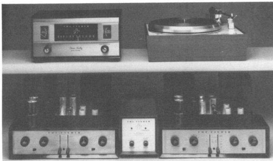
**EARLY HI-FI** - Top Shelf: Fisher FM 90X, 1957. The first of their famous "Gold Cascade" front ends, it also introduced the 6DJ8 tube to the U.S. market. Reko Kut Rondine 2 turntable (not affiliated with Fisher). Bottom Shelf: At center is an MPX 100 multiplex adapter (1962) flanked by a pair of 50C mono preamps driving a pair of 50A mono power amps (1952). (Stephen N. Raymer - Minneapolis, MN)
