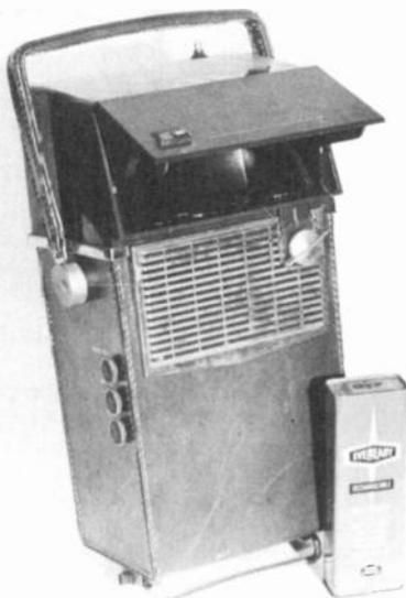
Figure 1. Philco Safari. First transistorized, portable TV. Rechargeable battery alongside.
