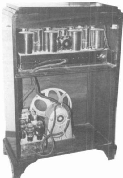
Figure 2. Rear view of Scott Allwave 15.
