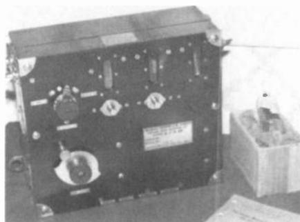
3-tube aircraft radio receiver, Model SCR-59, 1917-18, non-regenerative detector and two-stages of audio amplification. (George Potter)
