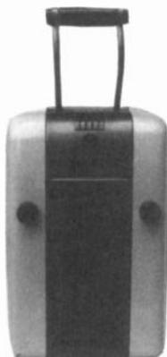
**WESTINGHOUSE MODEL H-126** - This 1948 model is similar to the 1946 version except that it used a 35L6 tube in the output stage instead of the usual 35A5. While Westinghouse called it their "Little Jewel," radio collectors often refer to it as the "refrigerator" model. The handle folds down and disappears behind the cabinet. (Doug Burskey - Mansfield, OH)
