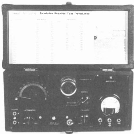
22.5-volt battery. It was discovered that the 30 tube would oscillate quite well at the low filament and plate voltages; thus, smaller batteries could be used.
