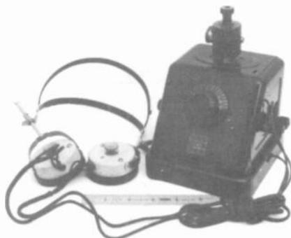
**TELEFUNKEN** - Crystal set (Rfe.6) of about 1928 vintage. Shown with F.R.I.H.O. detector and DTW headphones. A single variometer - single tuned circuit with very low "Q". Antenna taps for long wave and medium wave stations. Detector is extremely easy to operate. Binding posts on both sides allow parallel connections of two sets of phones. This set was exported to, and used in, Italy. It has a metal Italian radio license tag mounted to the back of the set. (Robert Lozier - Monroe, NC)
