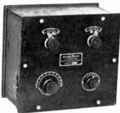
Figure 12. 2B tuning unit, panel view.
