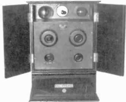
**GECOPHONE BC 2001** - This is a two-valve receiver manufactured in Great Britain in 1922, with bottom compartment for battery storage. (Greg Farmer - Fridley, MN)
