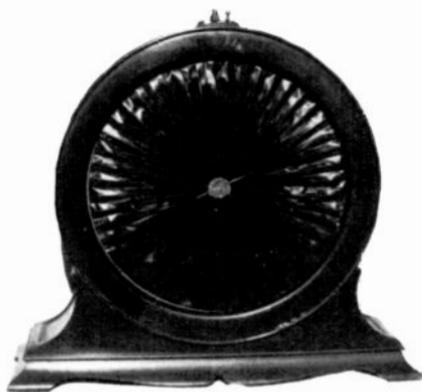
**VICTOR LUMIERE #1** - This is one of a few speakers produced worldwide that utilizes a pleated paper diaphragm to produce sound. This feature supposedly made the speaker more omni-directional. (Greg Farmer - Fridley, MN)
