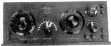
**UNUSUAL GREBE** - An early Model CR-5. The unique items are the exposed tube, surface-mounted rheostat, battery binding posts on the front panel, and lack of the thumbwheel controls which appear on the later model. The radio has no provision for turning off the "A" voltage. Inside, the variometer is made of wood instead of the bakelite as with the later model. (Bob Deuel - Ashland, OR)
