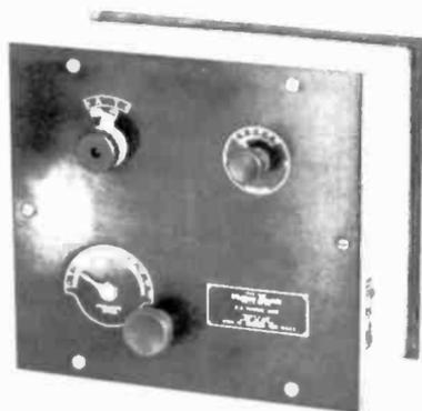
Figure 11. 2A tuning unit, panel view.
