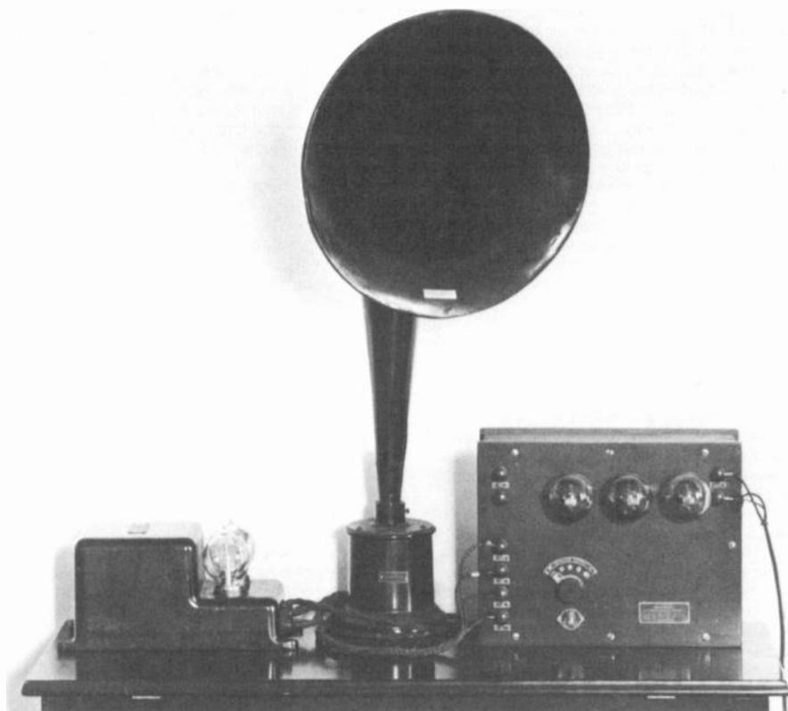
Figure 1. The No. 2A power supply and the No. 10A Loud Speaking Telephone Outfit consisting of the No. 7A two-stage A.F. amplifier and the No. 516-W horn.
