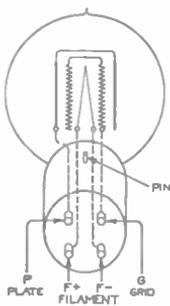
Diagram of a vacuum tube showing internal components and terminal connections. Labels include P (Plate), F+ (Filament positive), F- (Filament negative), and G (Grid). A 'PIN' label points to the top of the tube.
