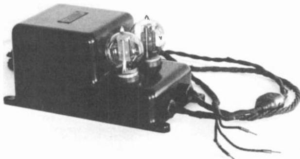
Figure 4. 2A power supply for the 7A amp. (Note: the 2A uses two type 217A rectifier tubes; the critical eye will notice that the rear tube in this photo is a type 216A inserted for appearance since a type 217A was not available.)
