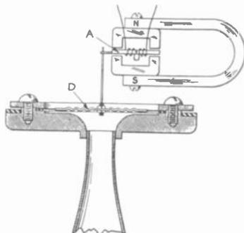
Figure 5. Driver assembly for the 516-W horn.
