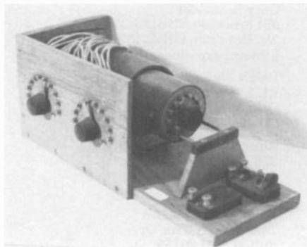
**HOME BREW LOOSE COUPLER CRYSTAL SET WITH PHONE CONDENSER** - Someone made this set in 1924, and it is a fine copy of the "Navy Type" coupler with tens and unit taps on the coil. The oak case is nice too. (Walter V. Worth - Wollaston, MA)
