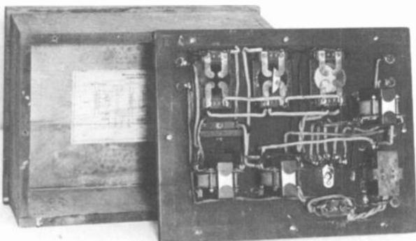
Figure 3. 7A amplifier, inside view.
