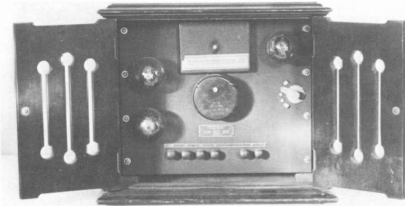
Figure 7. 14A amplifier-speaker, rear view.
