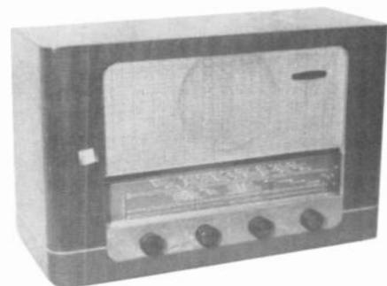
**PYE ENGLISH 8-BAND TUBE TYPE SET** - This set is very easy to tune, and has exceptional tone. Manufactured in 1939, it has an excellent method of band switching and even has a "ground" position. (Walter V. Worth - Wollaston, MA)
