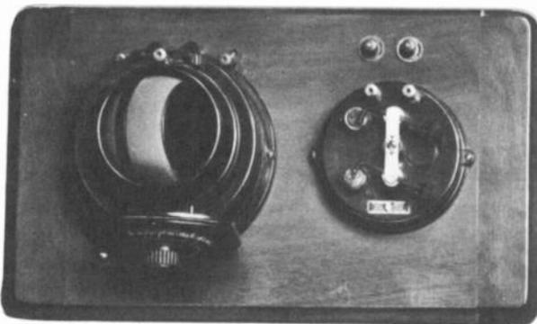
Figure 2. Atwater Kent Crystal Set with Type 11 Tuner.
