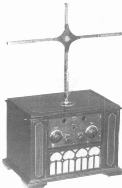
**DEFOREST D12** - This rather large 1924 set used an internally-mounted catwhisker and crystal for detection along with a four-tube circuit for power. Later versions substituted a detector tube instead of the crystal for ease of operation. (Dave Crocker - Lyndonville, VT)
