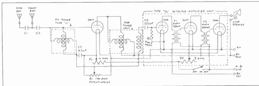
Figure 2. Schematic Diagram of Atwater Kent Model 9A
