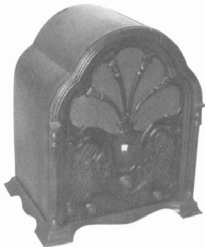
**FADA CATHEDRAL** - This Model 43 receiver was my 1000th radio! It has seven tubes, a TRF circuit with push/pull output. The front is of Repwood-type of material. (Ron Boucher - Goffstown, NH)
