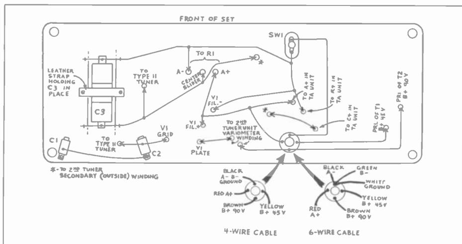
Figure 3. Bottom View of Breadboard and Battery Cable Hook-up for Atwater Kent Model 9A
