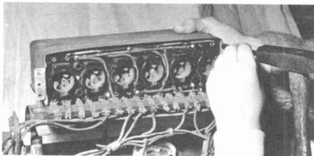
Figure 4. Tap the can on its edges using a bit of brass and a hammer.
