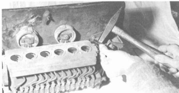
Figure 2. A single-edged razor and hammer is used to cut the seals.
