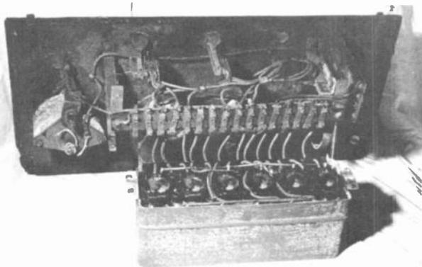
Figure 3. Tip the catacomb out for access.
