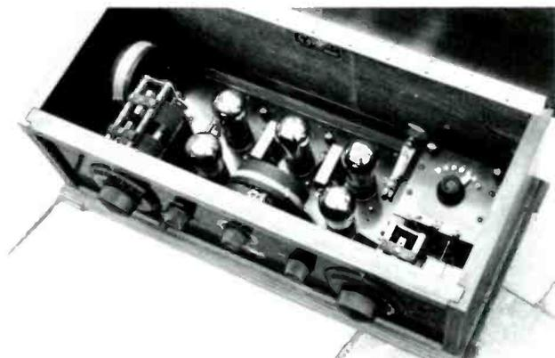
Figure 2. Interior view of the Oriole Model 7B showing the 5-tube layout and the unique antenna coil tap switch to the right.
