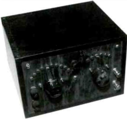
**LABELLE MODEL 21** - This dual-tapped crystal set was produced in 1923 by the Labelle Radio Co. of Attleboro, Mass. The panel is orange and black swirl to match the two tap switch knobs. The small center knob rotates the catwhisker on the crystal inside the box. *(William Key - Halifax, MA)*
