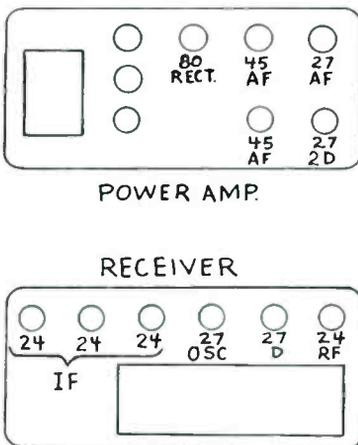
Figure 6. Tube layout of Victoreen Type A.
