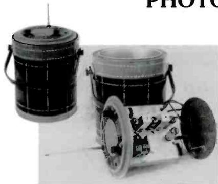
**PICNIC RADIO** - This Scottie Cooler radio is a four-tube novelty set. The receiver is hidden inside a plaid picnic cooler case with a telescoping antenna. No other manufacturer's information is available. (*Frank R. White - Olathe, KS*)
