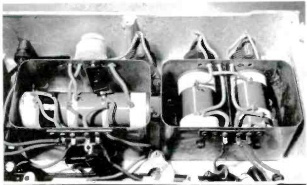
Figure 4. RF coils of Victoreen Type A with box covers removed.
