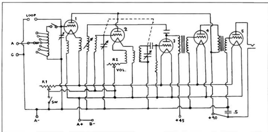
Figure 3. Schematic diagram for the Oriole Model 7B
