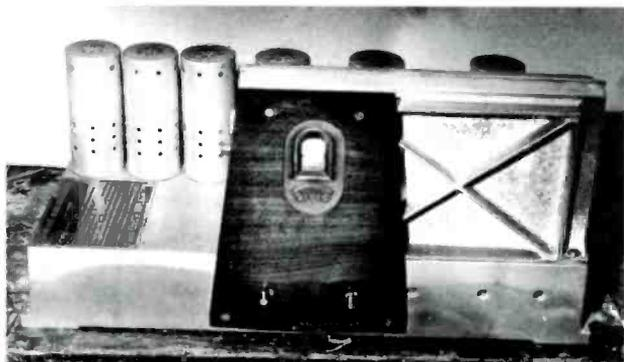
Figure 2. Front of Victoreen Type A chassis showing heavy aluminum casting.
