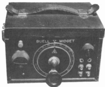
BUELL MIDGET - This very small set, covered with black leather, utilized three UV-199 tubes. This is actually a very well-made set. (Greg Farmer - Fridley, MN)
