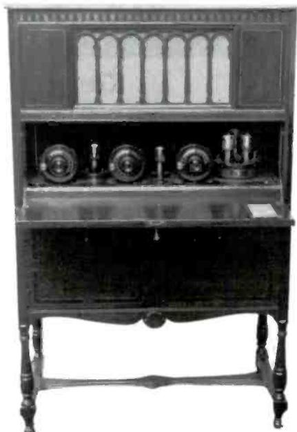
**BREADBOARD CONSOLE** – This is the Atwater Kent Model 1100 that was sold in a Pooley cabinet. It has a rectangular wooden horn speaker built into the top and a battery compartment below. (*George Found – Kitchener, Ontario, Canada*)
