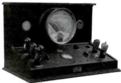
**VINTAGE TESTER** – This is a Jewell tube tester, Pattern 538. Approximate time of manufacture is the early 1930s, as it will not check tubes with more than five pins. It will accept those type tubes with grid caps. I paid \$16 for it in 1975. It is in very good condition, and I would like to know more about it. Does anyone have one? (*David Ringling – De Soto, MO*)
