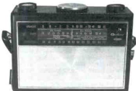
**MULTI-BAND PORTABLE** - The Wards Airline Model GTM-1233A was a three-band (BC, marine and SW) portable of the 1950s. The leather case slips off straight up to expose the chassis. It is an excellent SW performer, even today. (Bob Moore - Lakewood, CO)
