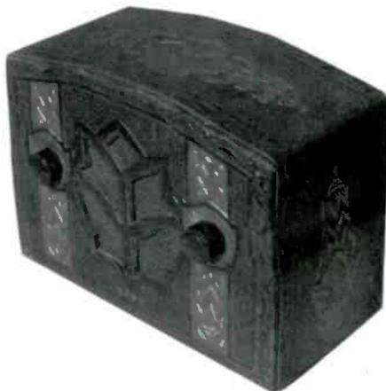
**BEST AC/DC** - The model number was missing, but the receiver was manufactured by the Le-Wol Corp. in 1934. Like the one pictured in *Flick of the Switch*, page 185, it is covered with an embossed leatherette, but instead of brown, this one is green with gold trim. The tubes are: 25Z5, 43, 6D6 and 6C6. (Dave Crocker - Lyndonville, VT)
