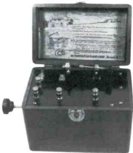
**THE LITTLE GIANT** - The Metropolitan Radio Corp., of Newark, New Jersey, made this Little Giant crystal set in 1922. The knob on the side moves a coil within another coil inside the cabinet. A slide switch selects 600 or 800 kHz. (Fred Geer - Jacksonville, FL)
