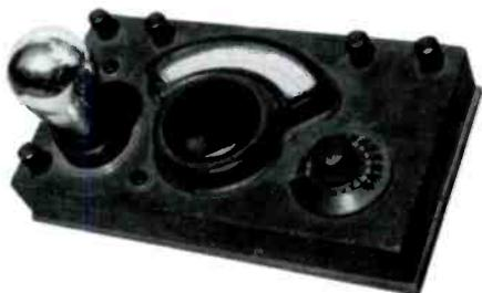
**EARLY TUBE TESTER** - This Hoyt Model 100 tester was manufactured by the Burton Rogers Company of Penacook, New Hampshire. Instructions on the bottom listed the limited number of tubes it would check as: WD-11, WD-12, UV-201, UV-301, C-299, UV-199, DV-3, WE-215A and UV-200. (Dave Crocker - Canton, MA)
