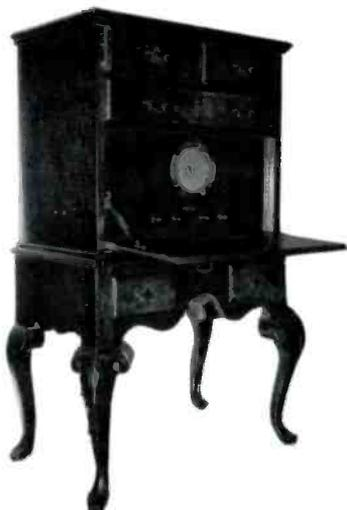
**RCA VICTOR** - This radio has a mahogany wood cabinet in a lowboy dresser style. The two top drawers can open, and the center panel drops to reveal the receiver's controls. The radio has four bands, but I cannot locate the model number. (David Masterson - Meriden, CT)
