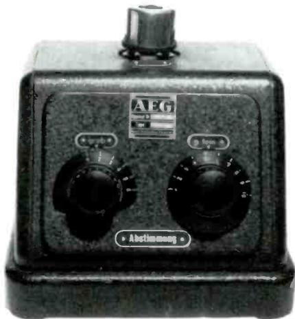
**GERMAN CRYSTAL SET** – The AEG Type D crystal receiver was produced in Germany before 1930. It has a metal case and uses double tuning controls. (Erwin Macho – Vienna, Austria)
