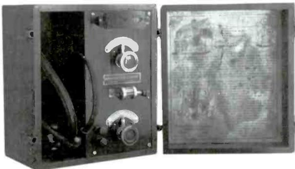
Figure 1. The Canadian version of the DeForest Everyman Crystal Set made by the Canadian Independent Telephone Co. of Toronto.
