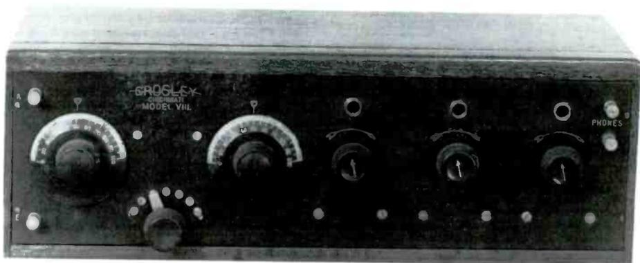
**CROSLLEY MODEL VIII** - This is a 1923 three-tube TRF receiver. The older style dial controls, the ground post scribed "E" (earth), and the period after the model number on the panel quickly identify it as an early production set. Inside are the early-type wood book tuning condensers and porcelain tube sockets. (Dave Crocker - Lyndonville, VT)
