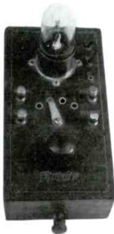
**STEINITE** - This is the Steinite Type 26-1 made by the Tri City Electric Supply Company. It is a one-tube regenerative receiver. (*Frank R. White - Olathe, KS*)
