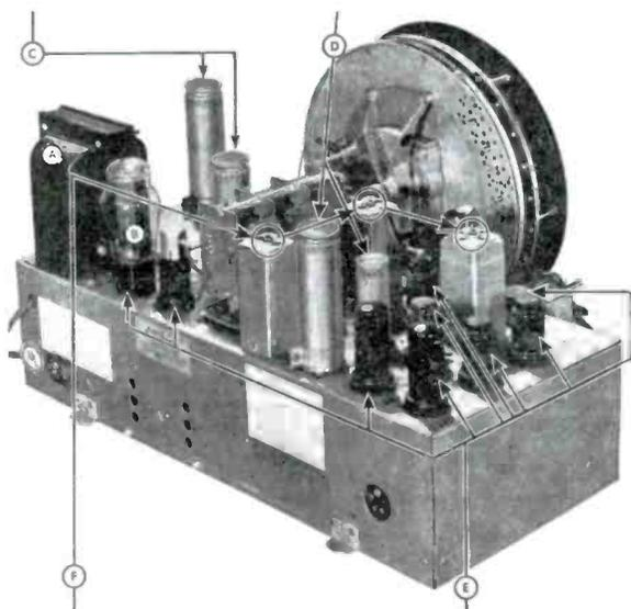
Figure 2. A Typical AC radio chassis with the filter capacitors, power transformer and rectifier tube identified. F = IF transformers, A = power transformer, B = rectifier tube, C & D = filter capacitors.
