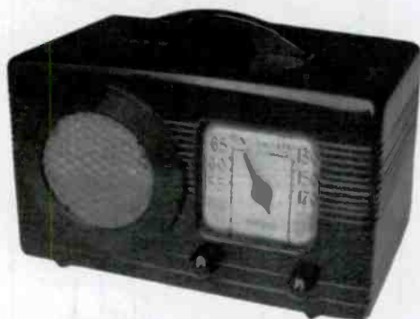
1940 MOTOROLA - The Model 50XC4 was an amber Catalin cabinet radio with a porthole-type speaker grille. The knobs are translucent. The five-tube set received the broadcast band only. (Ron Boucher - Goffstown, NH)
