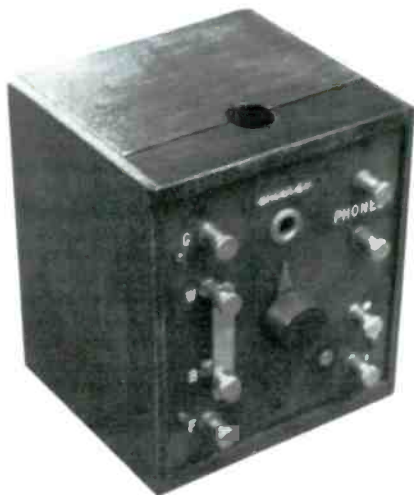
CROSLEY AUDION DETECTOR - This is the later, better designed, of two audion detector units offered by Crosley in 1922. It is often connected between the Crosley Model 1 crystal set and the Crosley RFTA tuner. (Dave Crocker - Duxbury, MA)
