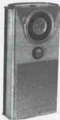
GE MODEL (?) - This General Electric transistor radio has a beautifully machined case. The antenna is beneath the black strip to the left. It has an earphone and RCA pin plug output jacks on the bottom of the case. The late 1950s would be my best guess as to its age. (Bob Moore - Lakewood, Co)
