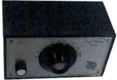
**MILLER TUNER** - The Miller Coil Co. produced this high fidelity tuner in 1956. It is a crystal set using sophisticated Miller coils which can separate stations better than most other sets on the market. It sold for \$14 in kit form or \$19 factory-built. (Fred Geer - Jacksonville, FL 32210)
