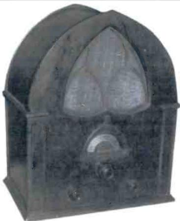
**AK CATHEDRAL** - In 1932, the Atwater Kent Radio Co. sold this table radio for \$69.50. It was advertised as a "compact" Model 84. It was a six-tube superheterodyne receiver. (William Key - Halifax, MA)
