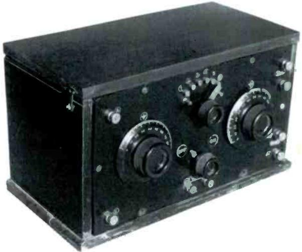
Figure 1. The Tuska Model 224 Receiver. Notice the small metal hooks used to hold the cover lid closed.
