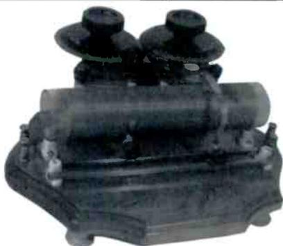
**UNIQUE HOME BREW** - This is a Hugo Gernsback Detektorium of 1910 design. The crystal is mounted in a cup that makes direct contact with the wire on the rather long coil, sliding up the coil for tuning. Another slider, on the left, controls the length of the coil. This unusual home brew tunes long wave and shortwave, and even today its owner claims it will pick up Radio Moscow and the BBC. (Fred Geer - Jacksonville, FL 32210)
