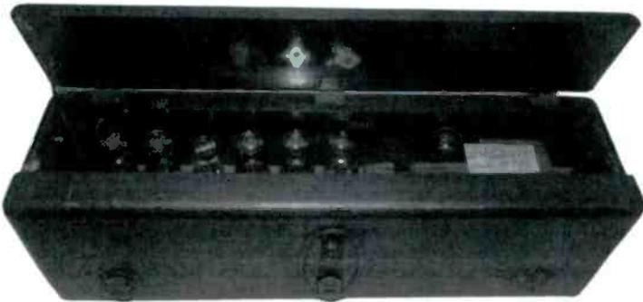
**RADIOLA 18** - The Radio Corporation of America (RCA) manufactured this AC receiver in 1927. It is a seven-tube TRF that sold for \$115. (Norm Landis - Kirkwood, MO)
