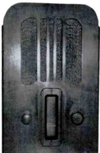
**STEWART WARNER** - This tombstone is a Model R-3043-A with the following tube complement: 6A8G, 6K7G, 6K6G, 5Y4G and 6Q7G, all of which are Arcturus blues. The unusual feature about this set is that the chassis is mounted vertically, and the dial is designed so that the set can be operated upright or on its side! It measures only 12 inches high. (Donald P. Amshay - Durham, NC)
