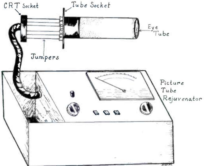
Figure 1. Setup for rejuvenating tuning eye tubes.
