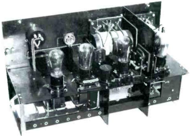
Figure 2. Rear view of the mystery set showing the chassis layout.
