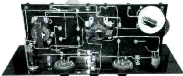
Figure 2. The Edison Model R-3 chassis viewed from below; the ketweweave coil is on the right and the crystal detector is at the bottom middle.
