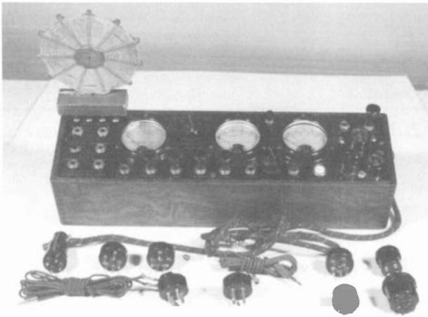
Figure 1. The Supreme 400A Diagonometer, shown with the various tube adapters and the Modulated Radiator (the oscillator coil located in the top left corner).
