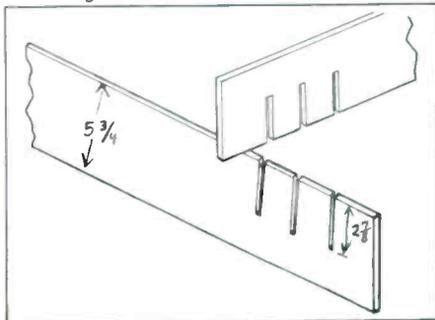
Figure 2. Alternating sections cut and ready for assembly.
