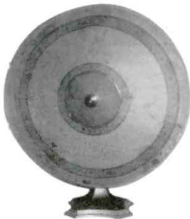
**WALCONE SPEAKER** - This is an eighteen-inch cone speaker made by Superior Radio Corp. of New York. It could be hung on a wall by the two hooks on the rear. The metal base is detachable. (Walter Worth - Wollaston, MA)
