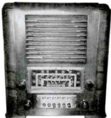
**CROSLY TABLE MODEL** - The broadcast band and shortwave receiver has an all-wood cabinet. It features push buttons for station tuning. The model number is unknown. (David Masterson - Meriden, CT)
