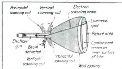
Figure 2. Basic diagram for magnetic deflection method. Reference: Donald Fink, *Principles of Television Engineering*, McGraw Hill, 1940, page 20.
