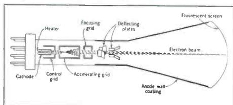
Figure 1. Basic diagram for electrostatic deflection method. Reference: Bernard Grob, *Basic Television, Principles and Servicing*, McGraw Hill, 1954, page 42.
