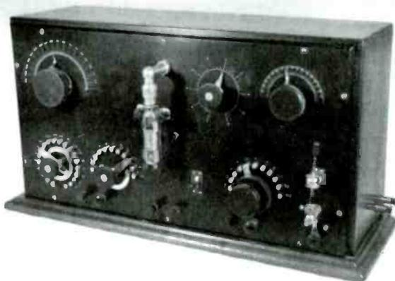
Figure 1. The audion tube receiver.
