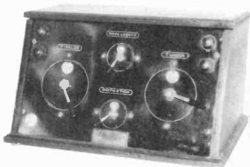
**MICHIGAN M10** - The Michigan Radio Corp. of Grand Rapids, Michigan, made this one-tube regenerative set in 1923. It is of very light construction with a formed aluminum panel and has room inside for A and B batteries. (Walter Worth - Wollaston, MA)
