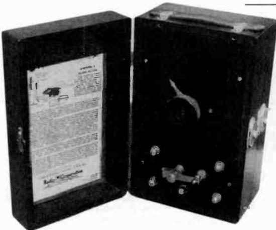
**RADIOLA I PORTABLE** - This is the Model ER-753A crystal receiver by RCA. The panel is stamped but not filled with a whitener, which makes it difficult to read. The rear compartment is for storage of Murdock headphones, which were recommended by RCA. The thin leather carrying strap is usually missing, and often the detector unit has been replaced by a more sensitive type. *(Dave Crocker - Duxbury, MA)*
