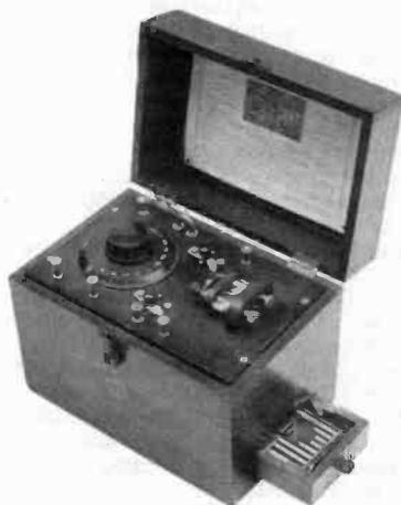
Figure 2. Another view of the Edison Bell Type B Crystal Set, showing battery compartment.
