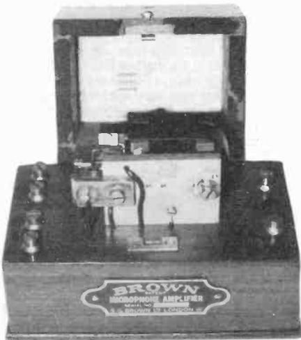
**BROWN MICROPHONE AMPLIFIER** - This is a one-stage microphone amplifier made by S. G. Brown Ltd. in 1923. It was designed so that several pairs of headphones could be used from a single crystal set. (Erwin Macho - Vienna, Austria)
