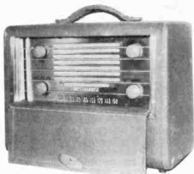
**WESTINGHOUSE 3-WAY PORTABLE** - This Model H165 in a brown leatherette case receives the AM band only. It operates on AC, DC, and battery power. Manufactured in 1937, the set is of high quality. (Walter Worth - Wollaston, MA)
