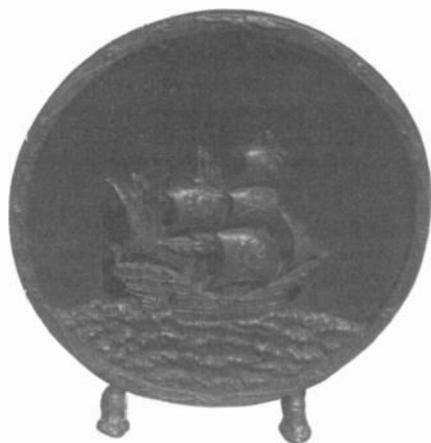
**TOWER "PIRATE SHIP" SPEAKER** - This early cone speaker was produced by Tower Mfg. Co. of Boston, Massachusetts. The frame and ship design is of heavy cast iron. This unusual piece appears to be in excellent condition. *(Doug Heimstead - Fridley, MN)*
