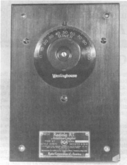
Figure 10. Front panel view of the Westinghouse Type RT antenna coupler. (Photo courtesy of Lauren Peckham)
