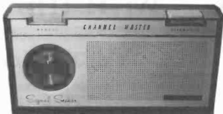
**CHANNEL MASTER SIGNAL SEEKER** - This ten-transistor radio features mechanical "seek" tuning, with a windup key on the back of the set. When you wind the key and press the automatic switch, the radio will search for the next available station. All the plastic components are aqua colored. The set comes with a fitted cowhide case with an earphone compartment. (Alan & Melanie Brooks - Seneca, SC)
