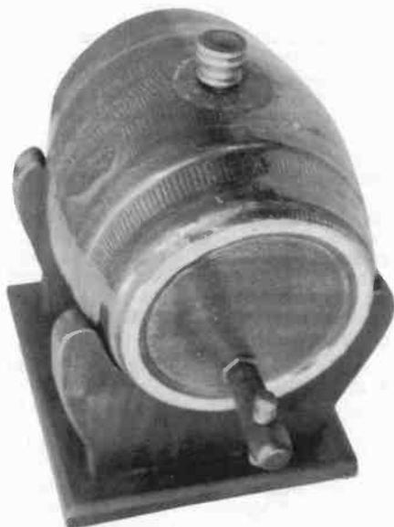
**RADIO DEVELOPMENT AND RESEARCH CO. MAGIC TONE** - This keg radio is in a ceramic, rather than wood, container. The spicket is actually the on/off switch and volume control, while the plug on top is the dial. (David McKenzie - Eustis, FL)
