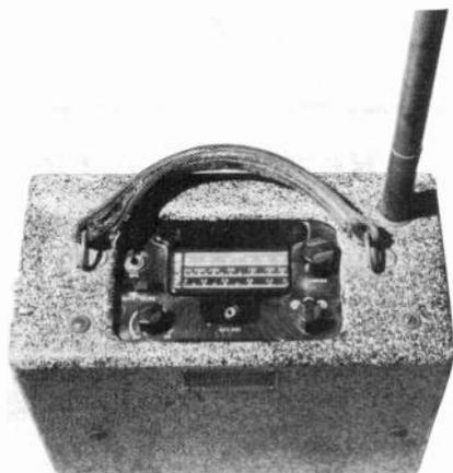
**LEARAVIAN RM 402 B BEACON, BROADCAST & AIRLINE RECEIVER** - This portable broadcast-aero band receiver has a nameplate on the front reading "The Pilots Preference." Made by Lear Avia Inc., Piqua, Ohio, this set covers the old air band of 200-400Kc, the standard broadcast band, and a 2-6Mc shortwave band. In the average home you could not fully extend the over ten-foot telescopic whip antenna. The hideous case, white with black painted spots, is original! (Allan H. Weiner - Yonkers, NY)
