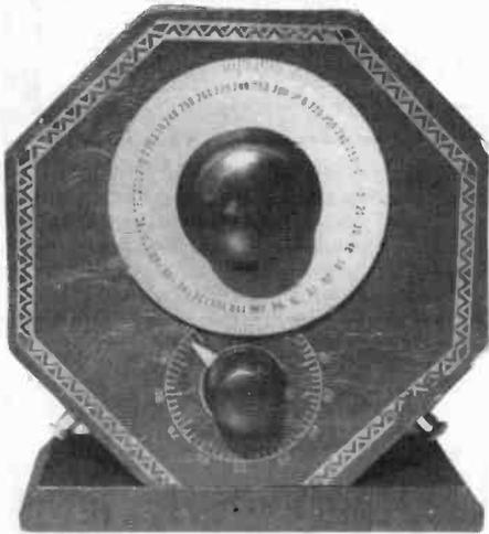
**ONE-TUBE RECEIVER** - This set, manufacturer unknown, has no visible tuning condenser! I had never seen a tuning arrangement like this and must admit it had me stumped for a bit. I was sure there had to be a condenser for tuning. The secret? When turned, the large, white round dial, on a threaded shaft, moves in and out from the face of the radio, thus acting as a variable condenser which changes the frequency. *(David McKenzie - Eustis, FL)*
