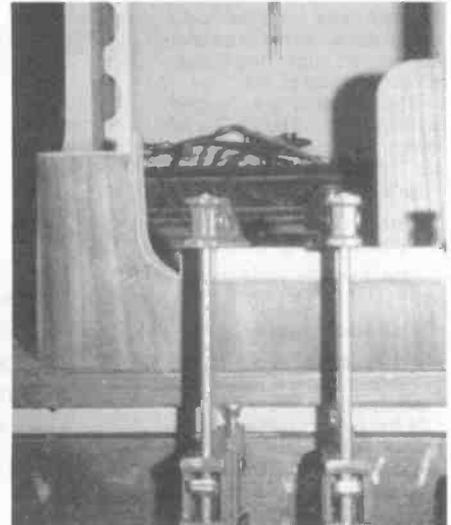
Figure 6. Another clamping method for holding the veneer on the borders of the speaker area.
