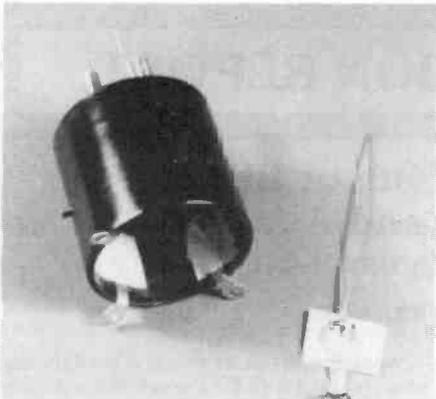
Figure 3. Solder lugs temporarily taped to the tube base.
