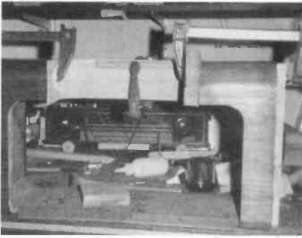
Figure 4. Clamps holding the glued veneer in place around the dial.
