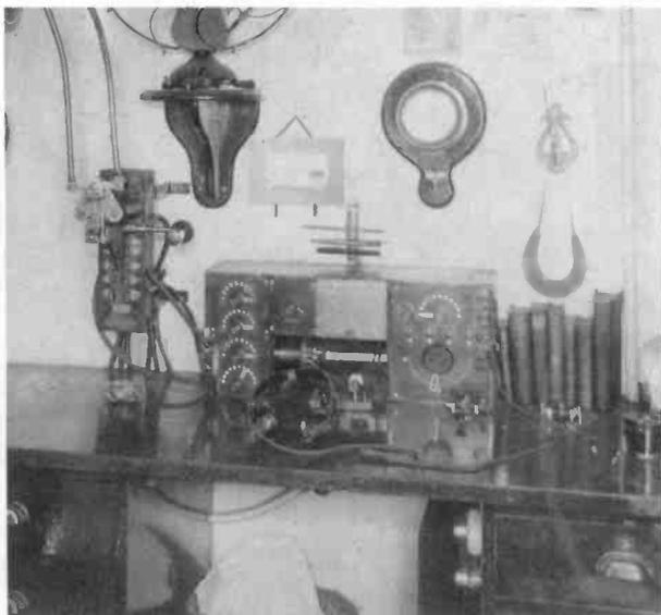
Figure 4. The I-P-76 tuner, which used a quenched gap spark transmitter, installed on the U.S.S. Nero. (This is an enlargement taken from our cover photograph.)
