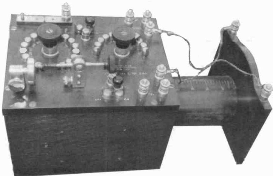
Figure 5. The I-P-111 receiver, also referred to as the I-P-76. (Photo from the collection of J. Kreuzer.)
