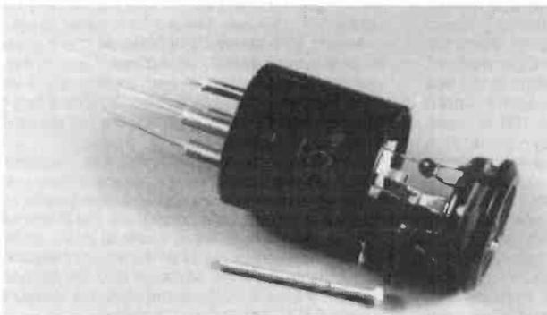
Figure 4. Bus wire threaded into each pin in the tube base.
