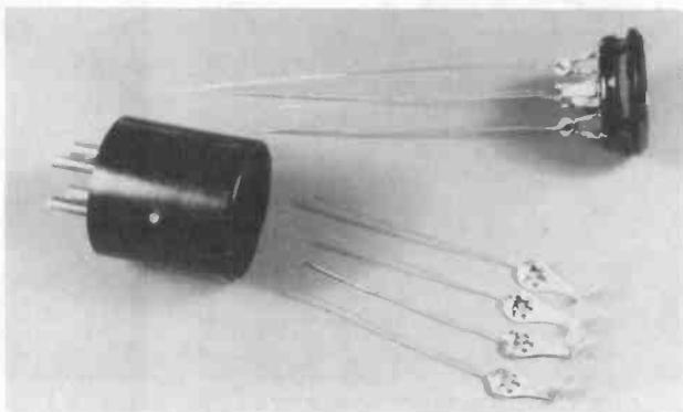
Figure 2. Four-pin test adapter components.
