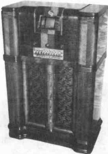
**MONTGOMERY-WARD AIRLINE MODEL 62-403-B** - This 1939 console has thirteen tubes and uses four Type 6F6 G tubes in push-pull for audio output. The movie dial screen projects the frequency (broadcast band to 22 Mc) on a lighted viewing screen. *(John Wieczorek - So. Bend, IN)*
