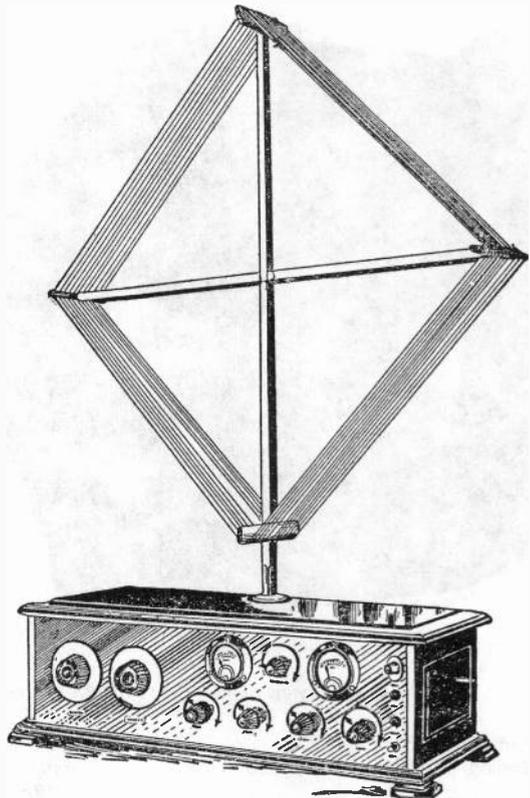
*Figure 2. Illustration from "Popular Mechanics" magazine showing how the completed set should look. Notice the loop plugged into the lid.*
