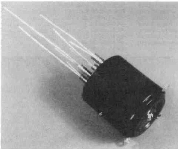
Figure 5. Two bus wires extending from each of the tube base pins.
