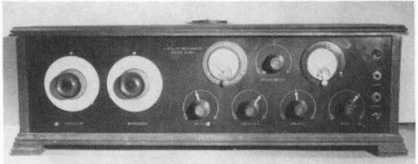
*Figure 1. The completed Popular Mechanics' Superheterodyne Eight receiver made from the factory kit.*
