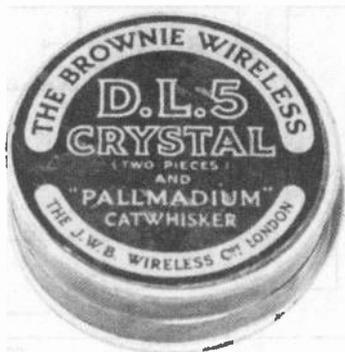
Figure 3. Pillbox container for replacement D.L.5 galena crystal and palladium cat's whisker.
