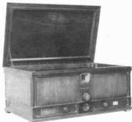
**STROMBERG-CARLSON 635A** - This 7-tube electric set has excellent shielding. It receives twenty stations utilizing its Model 11 wall speaker. The set has had no repairs; all parts are original from 1928. *(Walter Worth - Wollaston, MA)*
