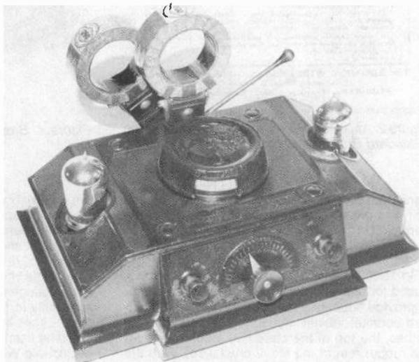
Figure 6. Brownie 2-valve receiver with Mullard dull-emitter type valves.
