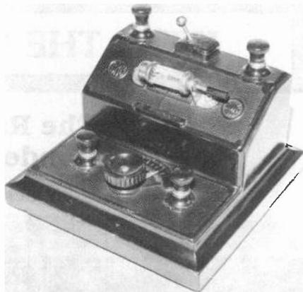
Figure 8. Brownie No. 3 crystal set. A wave-change switch replaces the plug-in coil of the No. 2.
