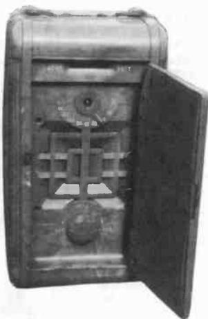
**GLOBE PORTABLE** - This small tube-type portable is an AC/DC model of the 1940s. It features a built-in antenna in the cover and looks somewhat like one of the popular cameras of that era. *(Ron Boucher - Goffstown, NH)*
