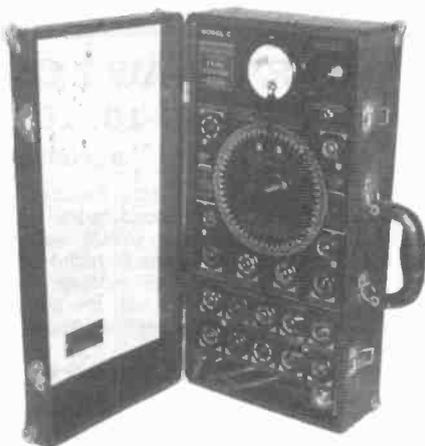
**CONFIDENCE AUTOMATIC TUBE TESTER, MODEL C** - Manufactured by Apparatus Design Co., this circa 1936 tube tester features tests for emissions and shorts, plus a pilot lamp test. The sockets are color coded and there are no switches, except for the 55-position rotary selector dial with a large Bakelite pointer. (Adam Schoolsky - Fremont, CA)
