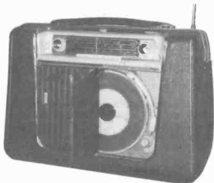
**METZ PORTABLE RADIO-PHONO** - This German-built radio from the late 1950s has three bands (SW, MW, LW) and a built-in 45 rpm turntable behind an opening front panel. The set works on battery or 110-240 volts and includes the original 2-prong German Mains plug. An album located inside the removable back panel holds ten 7-inch records. (Steve Kissinger - Thousand Oaks, CA)
