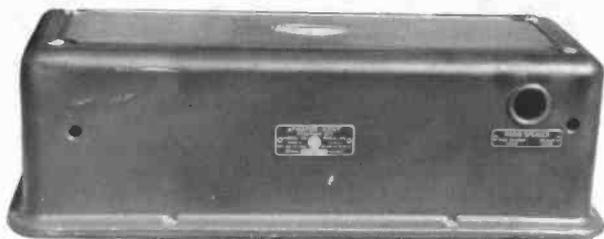
Figure 2. Rear view of the AK Model 35 showing the large loudspeaker connection hole and label.
