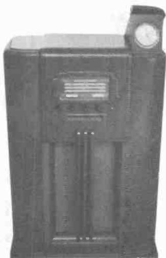
**GENERAL ELECTRIC MODEL G97** - Note the timer clock mounted in the upper right hand corner of the cabinet. This model has the AM band plus two shortwave bands. (Bill Graham - Aurora, NE)
