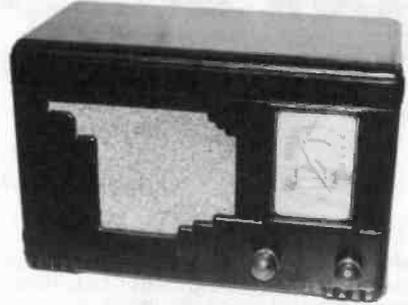
**SHELLEY RADIO CO.** - This "Commuter" radio, manufactured in Los Angeles, Ca., around 1937, features an Art Deco Bakelite front, but the rest of the cabinet is wood. The Golden Gate bridge and San Francisco Bay are drawn on the translucent celluloid dial. The grille cloth is not original. (Adam Schoolsky - Fremont, CA)
