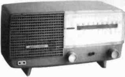
**SHARP MODEL UC228** - This Japanese set, probably from the early 1950s, uses miniature tubes and operates on the broadcast band and 3.98 to 12 Mc on the shortwave band. The nameplate on the left side says "Harpers." (Doyle Roberts - Clinton, AR)
