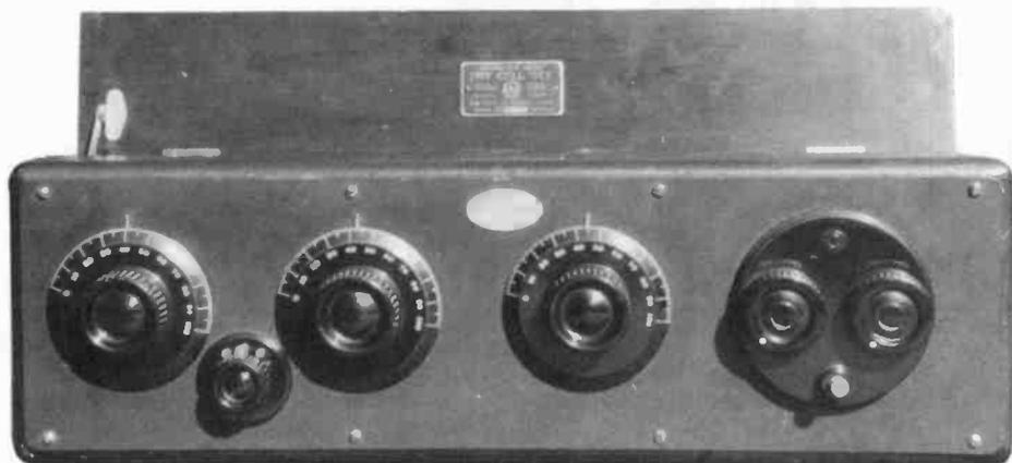
Figure 1. The Atwater Kent Model 21 dry cell set with the cover lid open to show the unique metal tag.
