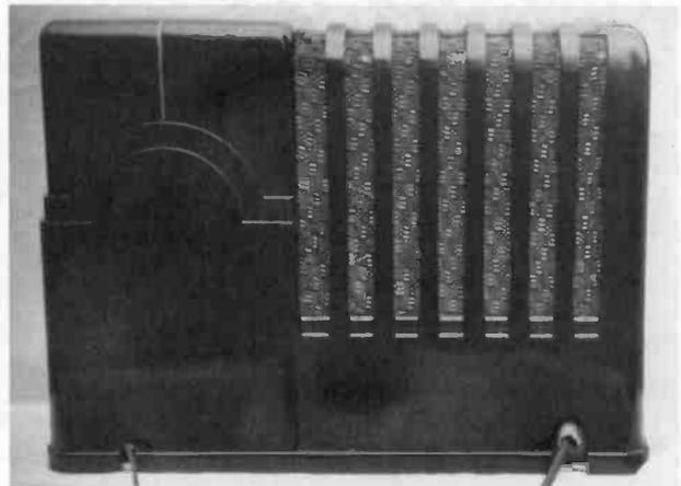
Figure 2. Rear view of the Model 4500. Note that the speaker grille wraps from the front of the radio across the top and down the back.
