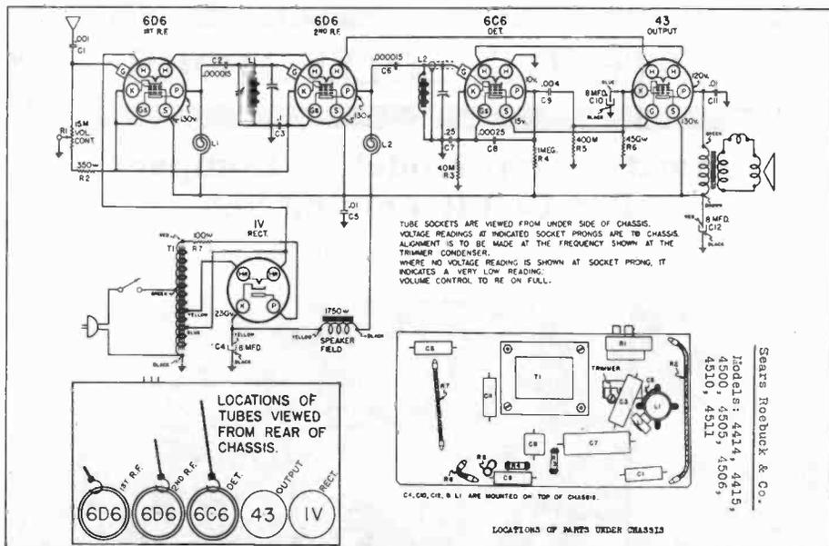
Figure 3. Schematic and parts layout from M. N. Beitman, "Most Often Needed Radio Diagrams, 1926-1938."
