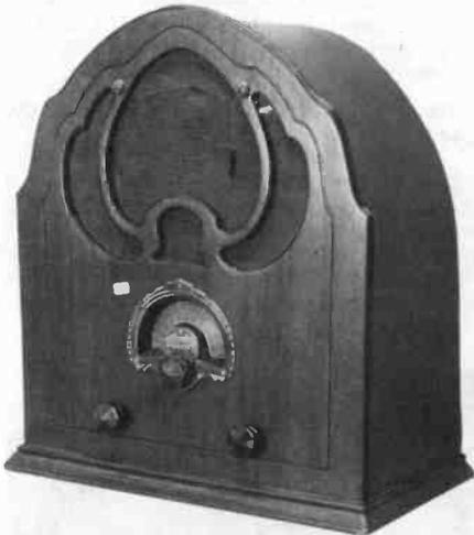
**VIKING CATHEDRAL** - This set resembles the style of the Ozarka Co. products. It has a 5-tube chassis of 1931 vintage and uses a projection of the needle on the dial face to indicate stations. Does anyone recognize the name of the manufacturer? (Walter V. Worth - Wollaston, MA)
