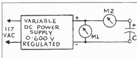
Figure 1. Equipment required for the reforming process: variable DC power supply, M1-voltmeter, M2-ammeter, C-capacitor.
