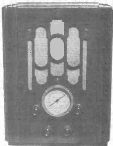
**ATWATER KENT MODEL 856** - Made in 1935, this set is an example of some of Atwater Kent's last products. It has 3 wave bands and uses 6 metal tubes and an 8" electro-dynamic speaker. *(Doug Burskey - Mansfield, OH)*
