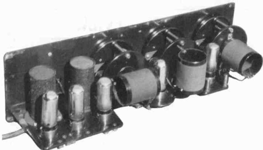
Figure 2. The chassis of the Atwater Kent Model 21. Note the UV 199 tube sockets and tubes.
