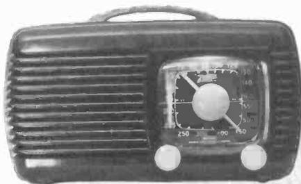
**ZENITH MODEL 6-D-510** - This brown Bakelite set was my first old radio, circa 1940. It uses the Zenith box-loop antenna with RF amplification via a 12J7-type tube. (*Colin Stump - Lancaster, OH*)
