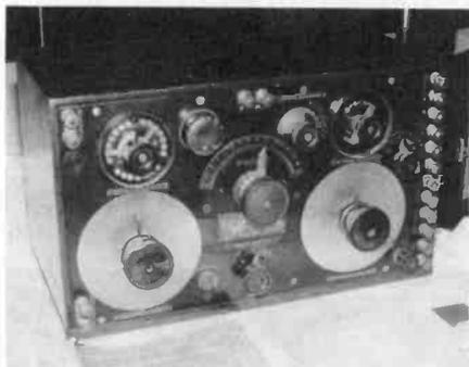
This Old Equipment Contest entry, a Marconi Model C294 C shortwave receiver operates either with a crystal or Audion detector.
