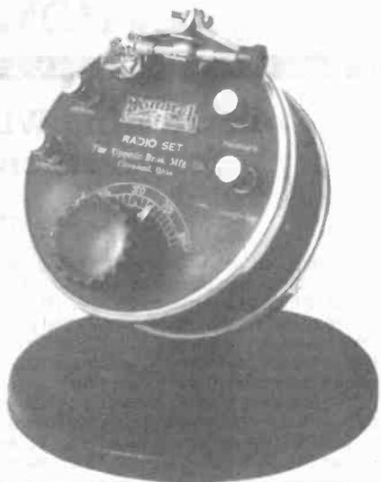
**MONARCH CRYSTAL SET** - This novelty set was made by the Rippner Bros. Manufacturing Company of Cleveland, Ohio. It has an open detector with 3 different crystals. (*Erwin Macha - Vienna, Austria*)
