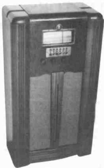
**AIRLINE (MONTGOMERY WARD) MODEL 62-370** - This 1938 floor model was found in a hayloft in "junkie" condition. The push-button, tuning-eye chassis works and has both broadcast and shortwave bands. (Doyle Roberts - Clinton, AR)
