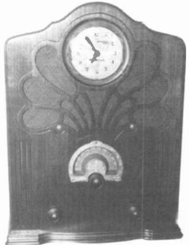
**BULOVA MODEL M-701** - A feature of this set is an adjustable timer to turn the radio on and off. This 1932, 7-tube, 175 Kc, IF model was purchased in poor condition at a farm auction in South Dakota. It still needs a glass and bezel for the clock. (Scott H. Timperley - LeMars, IA)
