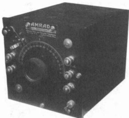
**AMRAD TYPE E CRYSTAL SET** - This set does not have the magnetic type detector, which may mean it is an older model. Note the detector in the lower right-hand corner. I also have the matching amplifier. (*Paul Giganti - San Carlos, CA*)
