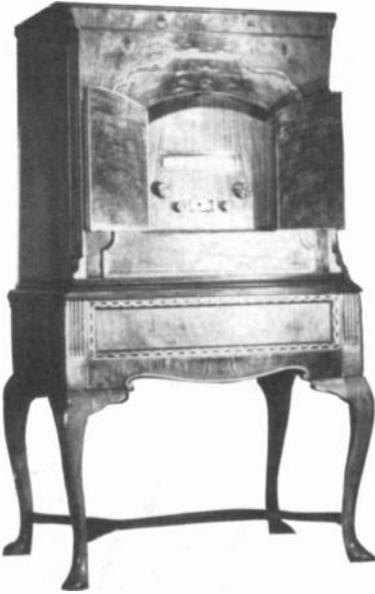
**GENERAL MOTORS MODEL 150** – The woods used in this floor model are exceptional! This 1930 TRF set has eight tubes. The speaker faces the floor and a phonograph is revealed when the top is lifted. (Kurt Thompson - Jacksonville, FL)
